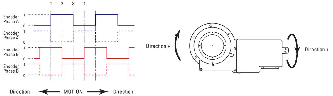
The incremental sensor consists of an optical scale and an encoder head. When the carriage moves, the encoder head generates square signals in quadrature and sends to pins #6, #7, #13 and #14 of the SUB-D15 connector.
